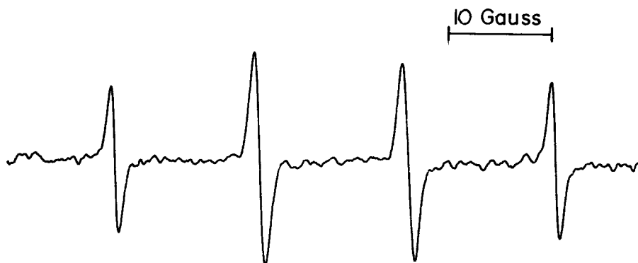
Fig. 2. The first derivative ESR spectrum of t -butyl hydronitroxide obtained upon reduction of MNP with microsomes and NADPH-generating system. The incubation mixture consisted of 0.02 M MNP in a Tris buffer (0.15 M) pH 7.5, 4 mg/ml microsomal protein 3.6 mg/ml glucose-6-phosphate, 0.66 mg/ml \text{NADP}^+ and 1.32 units/ml of glucose-6-phosphate dehydrogenase.
